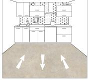
For most all-over designs, alternate sheets should be installed in opposite directions. Check design specifications before you start.
